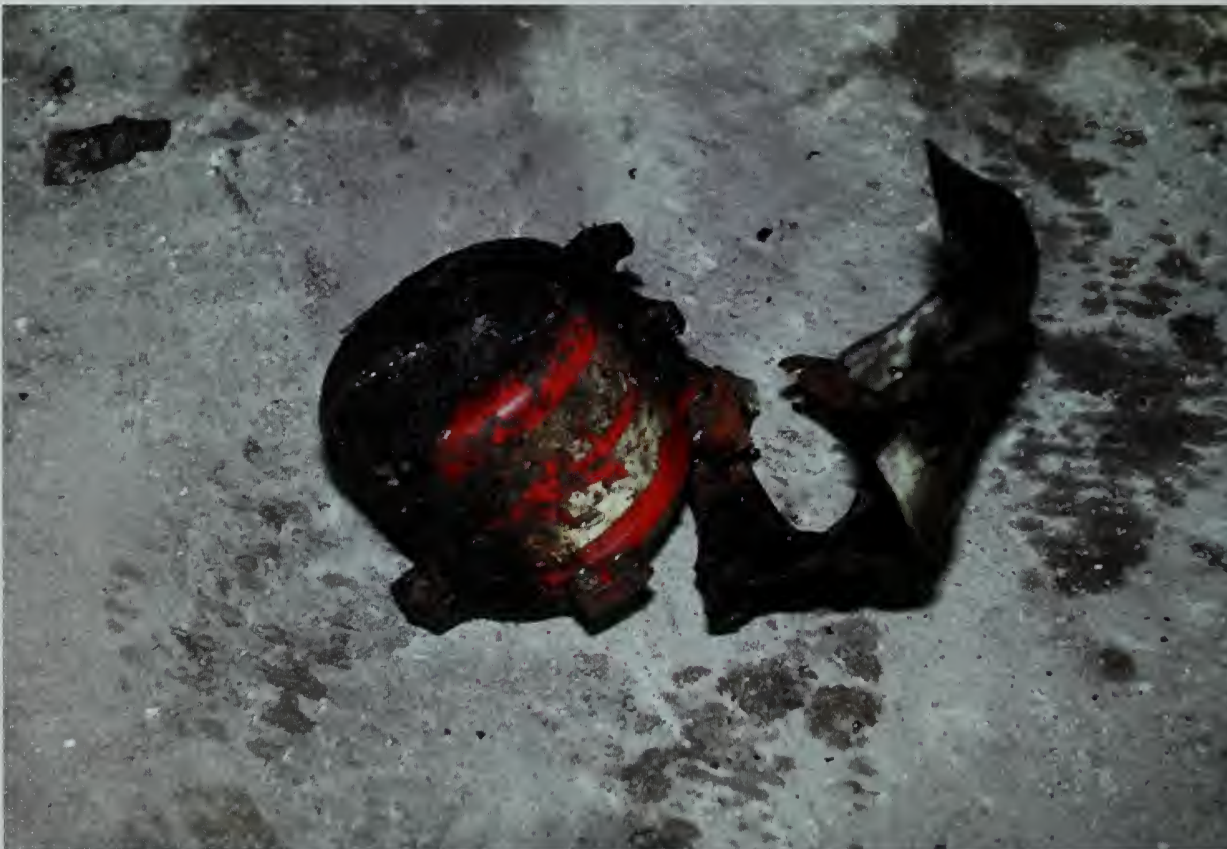
Flight data recorder found in the building near the hole in the inner C Ring wall leading to A-E Drive.
